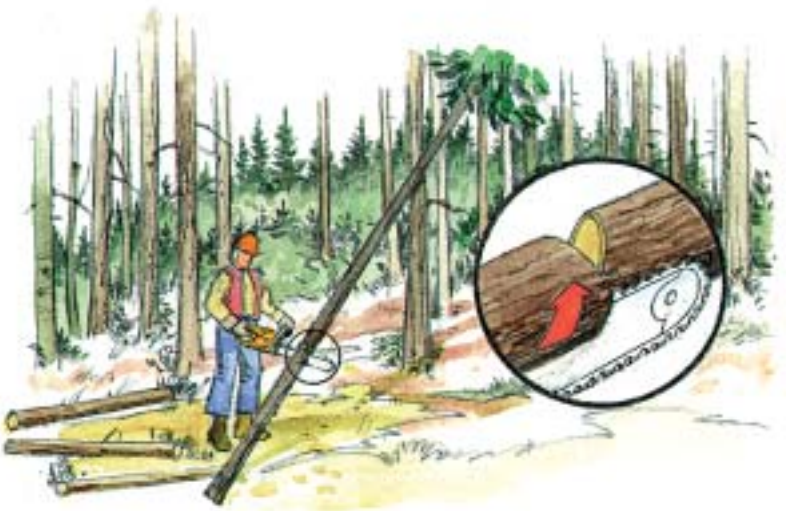
Proper method of blocking tree down
