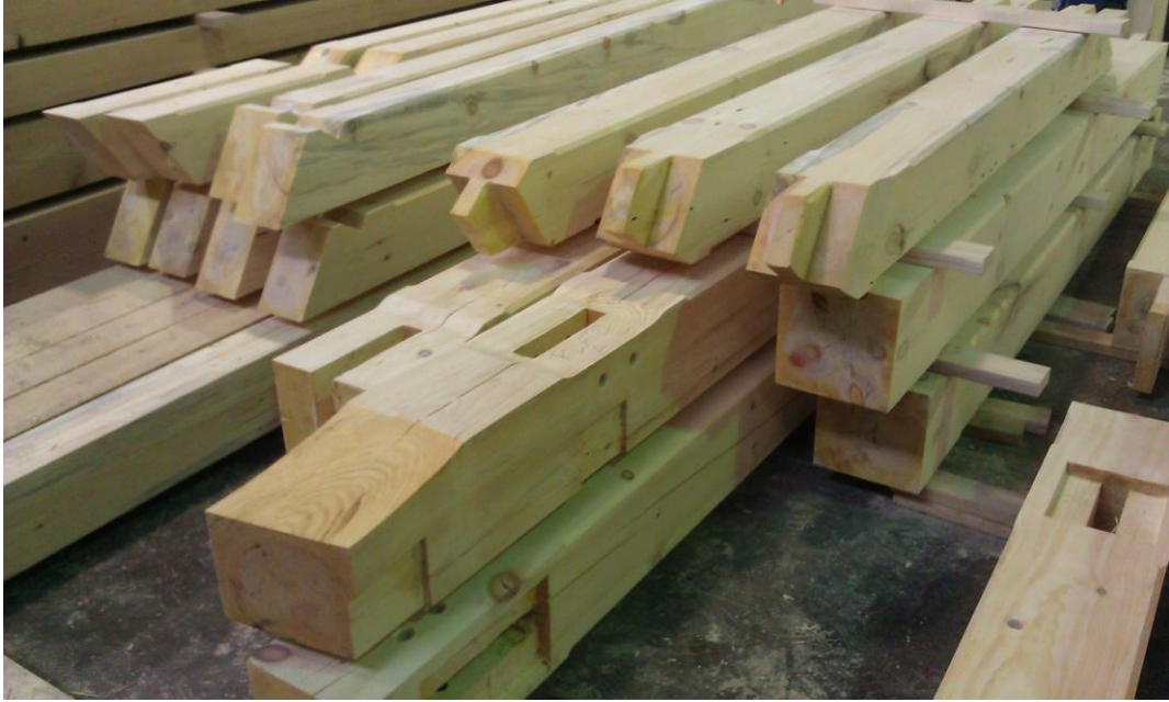
Timbers Stacked; Ready for Test Fit Up
