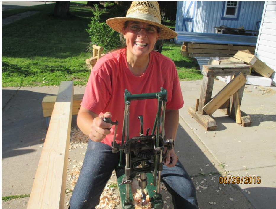
Drilling Mortises with a Boring Machine
