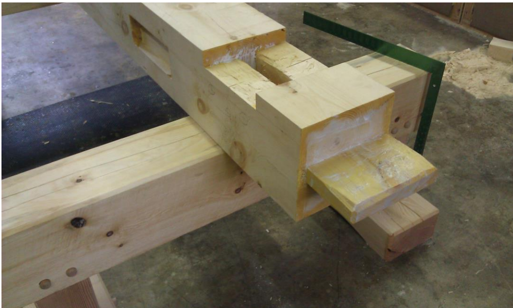
Post (tenon, mortise, and housing)
