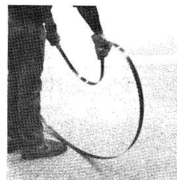
FIGURE B-9. BLADE INVERTING STEP #2.
