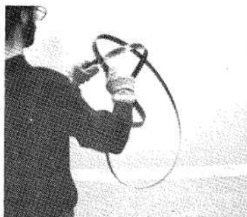
FIGURE B-6. BLADE UNCOILING STEP #3.
