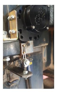
The cable should be always be 90 degrees out of the sensor.
