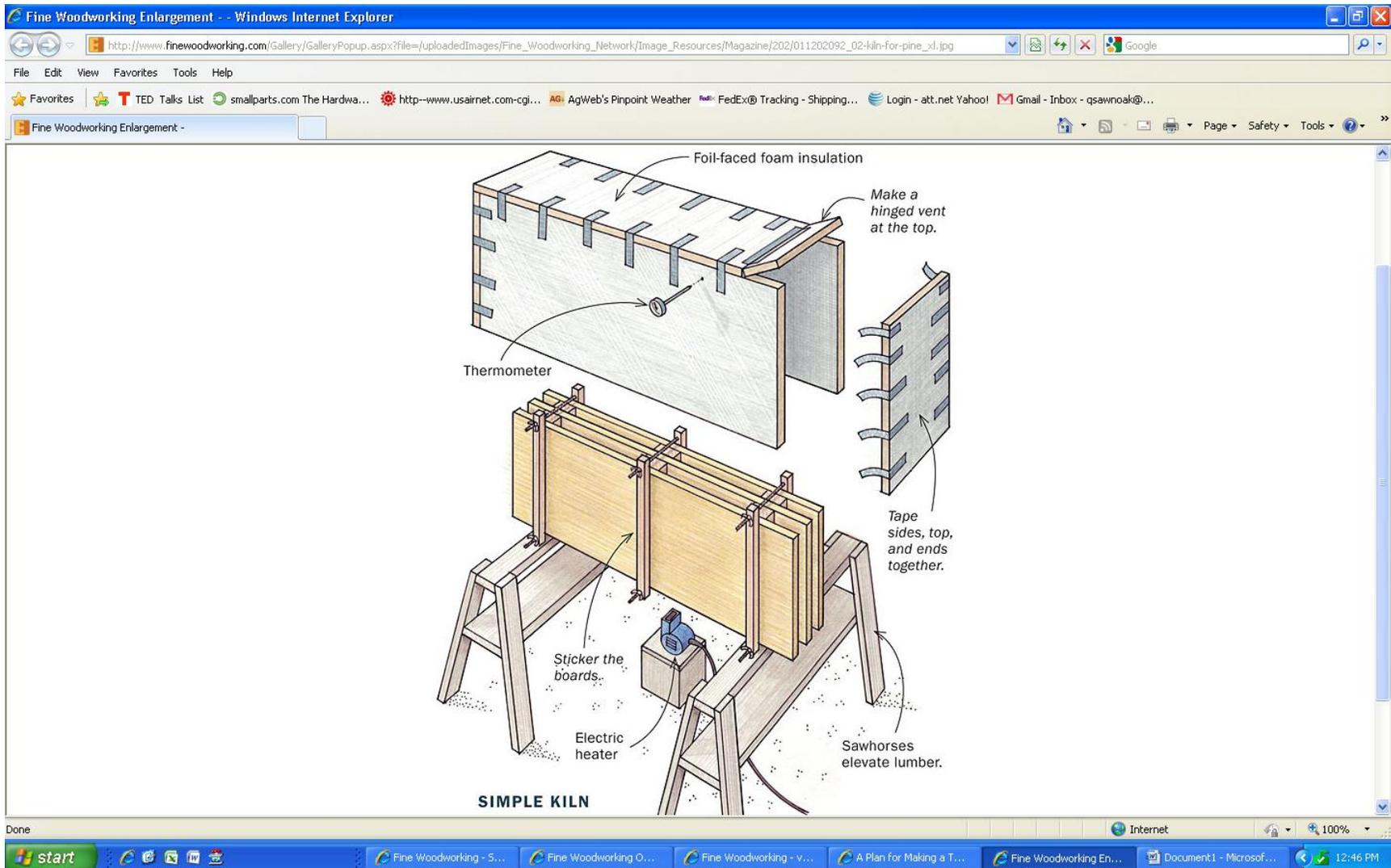
For larger pieces, FWW contributor Becksvoort makes a temporary kiln from foil-faced foam insulation. It has two sides, two ends, and a top, but no bottom. Make a hinged vent at the top of one end by cutting off a 6-in.-wide strip and reattaching it with tape.
