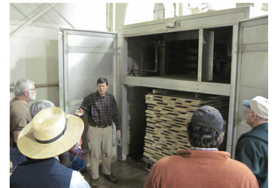
Millwork products require kiln drying for proper service
