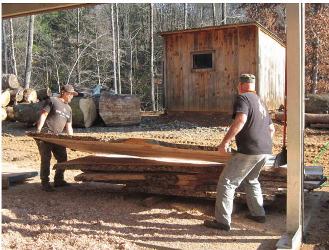
Manually moving live edge slabs after sawing
